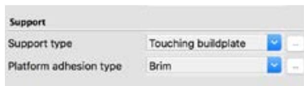
Select the support structure you would like for your print. A model will need supports if it contains overhanging sections as these will droop or fail to print without support. You can choose from “Touching build plate” which will put supports in wherever there is nothing between your overhang and the build plate and “Everywhere” which will also put supports in where your model overhangs itself.
