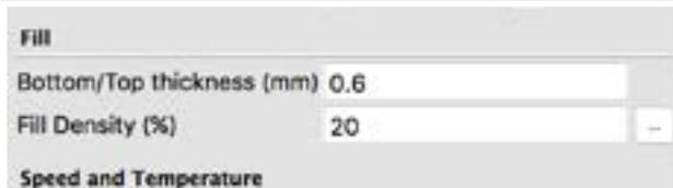
Most 3D models we download or draw in CAD are solid shapes. When it comes to printing a model, filling the whole of the inside of an object can increase the print time dramatically. For this reason Cura makes it easy to make your object hollow, there are two variables you can set to change how hollow your print is.
