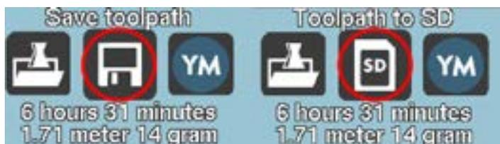
Once the card is inserted the Save toolpath button in Cura will change from saving locally to saving to the card.
