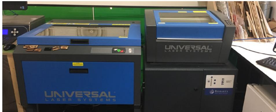
We have two laser cutters you can use to cut, score or engrave a range of materials. Materials you can work with:
